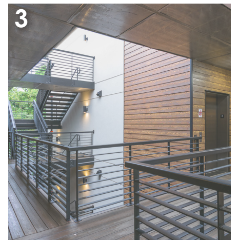
STEEL RAILINGS PAINTED BM163- "MIDNIGHT OIL" WITH WOOD RAILINGS STAINED TO MATCH DECKING
