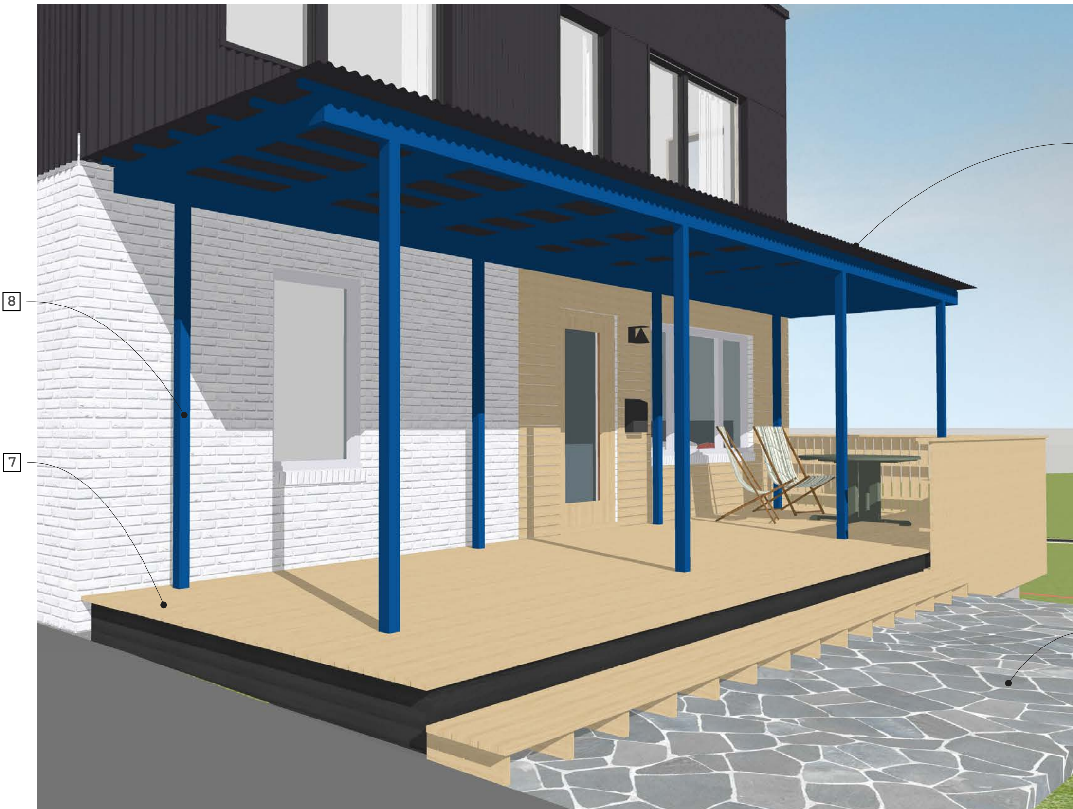
Metal porch structure painted color similar to Pantone 280C 3" square tube steel posts, 3x6 tube steel beams, 1 1/2" sq. purlins (pending structural review)
